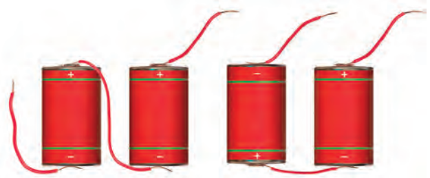
Fig. 10.2 (a) A battery of two cells (b) A battery of four cells
